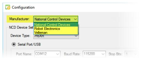
Quick Timer R2X supports relay boards of **National Control Devices**, **Robot Electronics**, and **Velleman** only for now.
