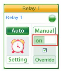
Click the switch button on the Control Panel for each relay channel to turn on/off single relay.
